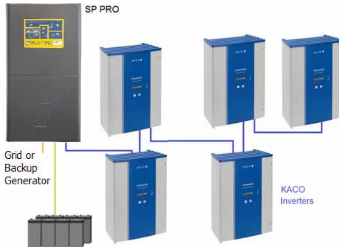
RS485 wired communications links between SP PRO and KACO inverters
